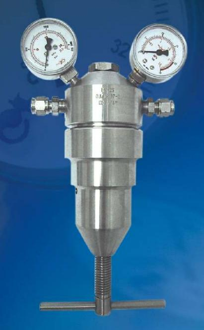
ROBUST REGULATOR WITH STAINLESS STEEL MEMBRANE (HP-25) SENSING ELEMENT OR PISTON (HP-50, 100, 200) (IN BRASS OR SS) DESIGNED TO ASSOCIATE HIGH FLOW RATES WITH HIGH PRESSURES IN HEAVY SERVICES, WITH BUILT-IN RELIEF VALVE.
