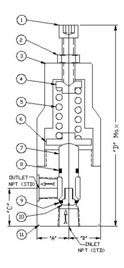
RVC-05 Soft Seated Relef Valve Threaded NPT Connections
