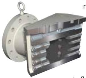
It is equivalent to having two four-path flow meters in one meter body. Cameron has conducted extensive research and testing to demonstrate that the four paths in any one plane can effectively determine the flow rate by averaging the four chordal path velocities, resolving any effects due to flow profile asymmetry.
