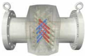
Fluid velocity measurements are averaged over the eight chordal paths of the two combined planes. Swirl effects in one plane will be equal but opposite in magnitude to the effects in the second plane. Averaging the velocity measurements has a net result of resolving any effects due to swirl on the overall measurement.
