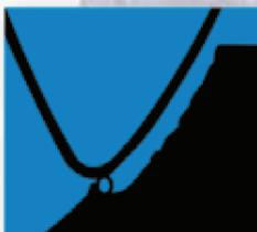
**Ordinary Seals** are damaged during shutoff. As flow is squeezed through fine-line opening, foreign particles are trapped. Complete shutoff grinds them into the seal. Results: premature damage, leakage, valve failure.
