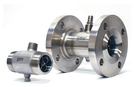
BARTON® Model 7400 Precision Turbine Flow Meters are designed for gas service in a wide range of industrial, commercial, pipeline and aerospace applications. Because the output from the pickup coil is digital, Model 7400 meters are an excellent match for electronic output devices — no analog to digital conversion is required. The rotor response is in milliseconds, providing precise metering in applications with rapidly changing flow patterns.
