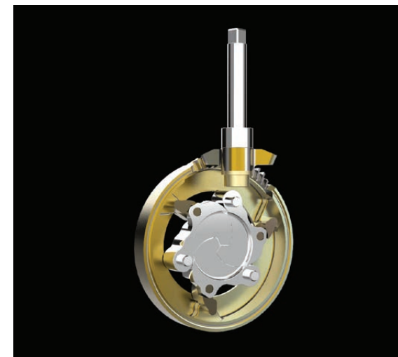
Figure 1: The Ring Gear enables the Dilating Disk™ Valve to deliver precise throttling and tight shutoff, with quarter-turn operation and low torque requirements. A Pinion Gear (top) transfers torque from the Valve Stem to the Ring Gear. The Ring Gear then drives the open/close motion of three interlocking Petals of the Dilating Disk™ Valve via three control Arms.
