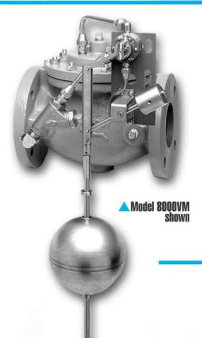
The OCV Series 8000 float control valves are designed to maintain a desired level in a tank or reservoir by opening for filling the tank when fluid is below the high level point and closing tightly when the desired level is reached.
