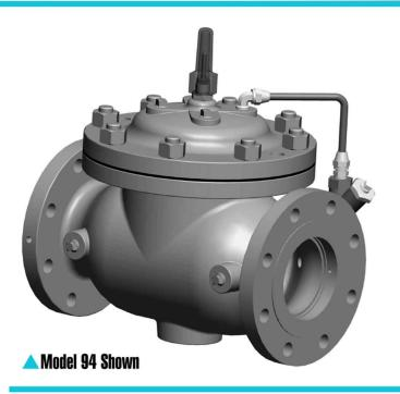
The OCV Series 94 check valve is a simple on-off valve that opens to allow forward flow when inlet pressure exceeds outlet and closes tightly to prevent backflow when outlet pressure exceeds inlet pressure.
